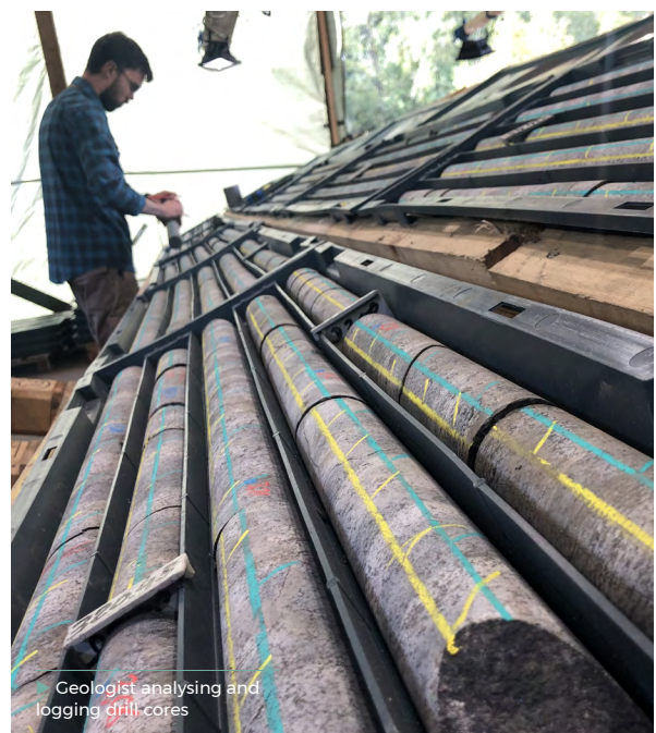
Example of a drill core. The dark colours could indicate a higher grade of ilmenite and magnetite
